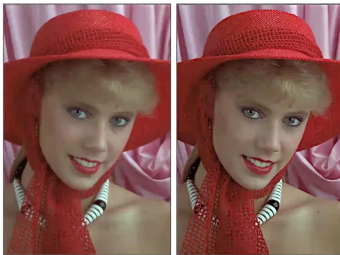
Original H.264 encoded QP=42 MS-SSIM=0.9275
