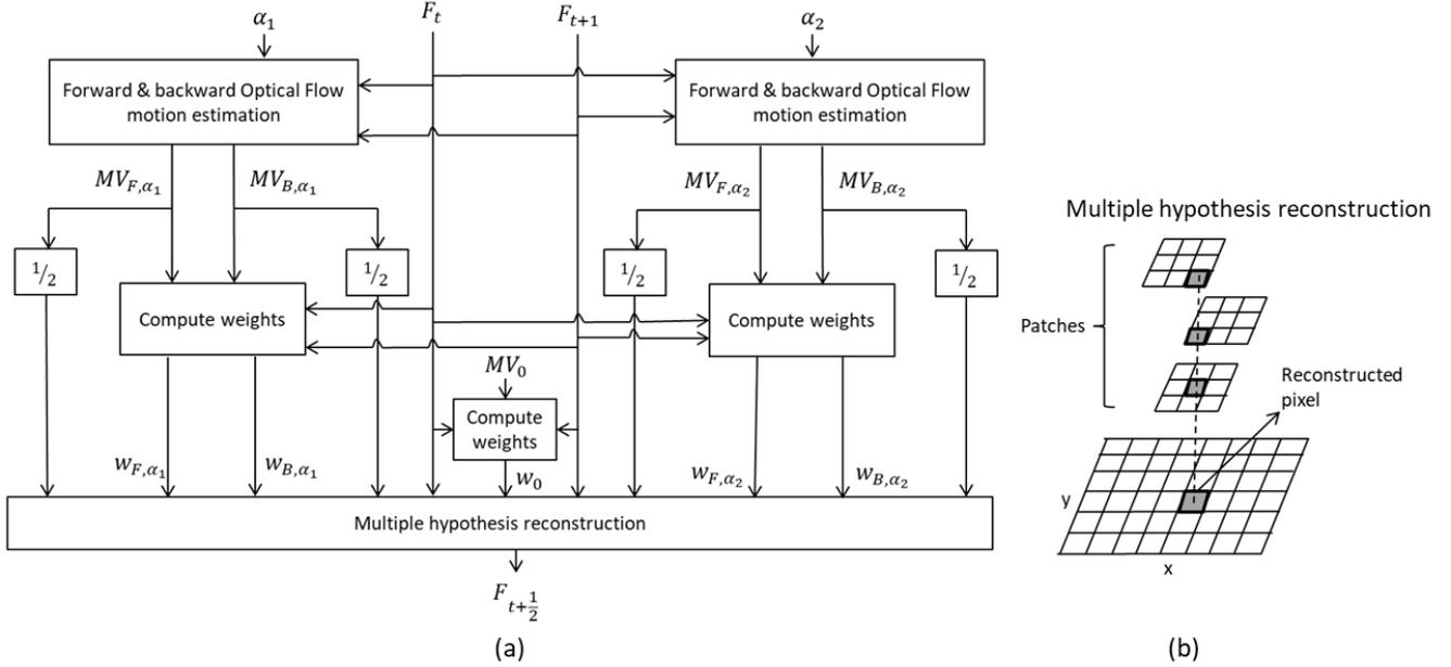
**Figure 1.** (a) Architecture of the proposed FRUC method. (b) Illustration of multiple hypothesis reconstruction.
