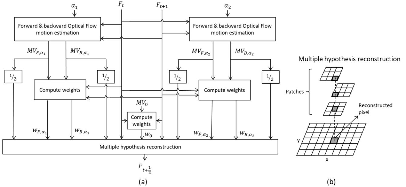
**Figure 1.** (a) Architecture of the proposed FRUC method. (b) Illustration of multiple hypothesis reconstruction.
