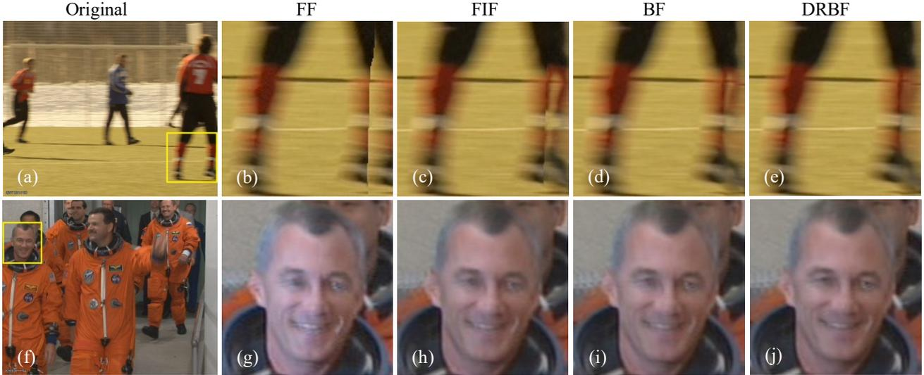
**Figure 2.** Visual quality comparison of the proposed FRUC schemes: FF, FIF, BF, and DRBF. (a) The 278<sup>th</sup> frame of the soccer sequence, and (b) – (e) are sections from the interpolated frames. (f) The 290<sup>th</sup> frame of the crew sequence, and (g) – (j) are sections from the interpolated frames.
